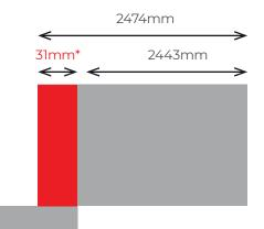
\* Note 31mm goes behind back of booth on full panel and fabric where they join in corners left or right sides.
